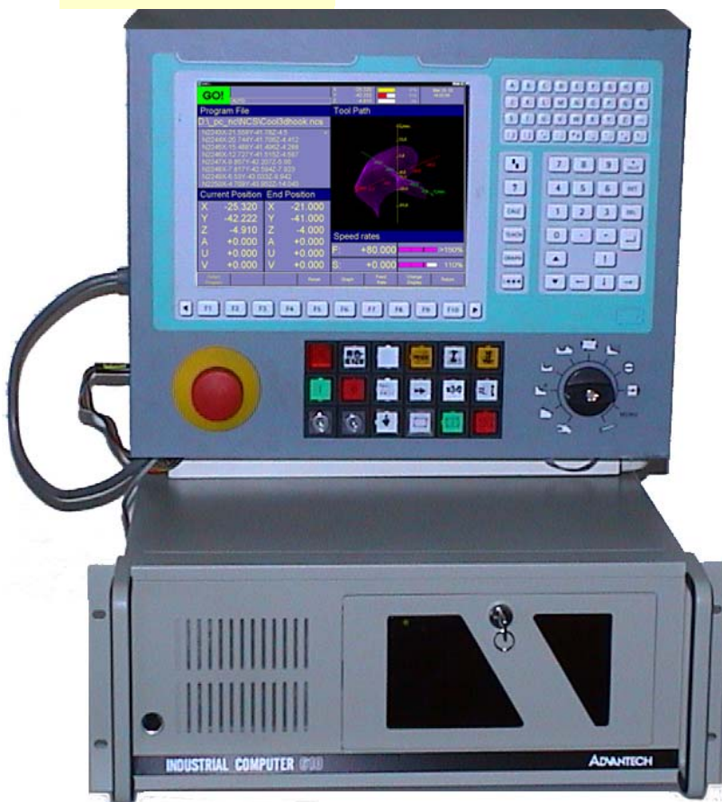
Pic. 1. WinPCNC numerical control system
